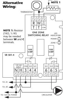
**NOTE 2:** When using Alternative Wiring diagram, the boiler operating control's ZC terminal will see the load of the circulator(s).
