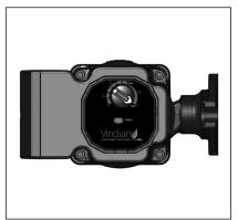
Position electrical junction box at 9 o'clock position for best programming and viewing orientation. Casing may be rotated to change flow direction. Locate the arrow on the casing body to determine flow direction.
