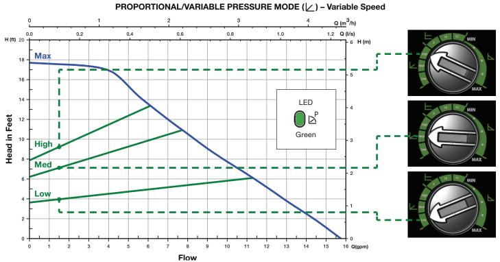
In Proportional/variable pressure mode ( $\not$ \_), the circulator maintains a proportional pressure differential ( $\triangle p$ -v) as heating load increases or decreases. Flow will change in relationship to the change in pressure differential. Selection options are Low, Medium, or High. If unsure on proper setting, select Medium and adjust as needed.
