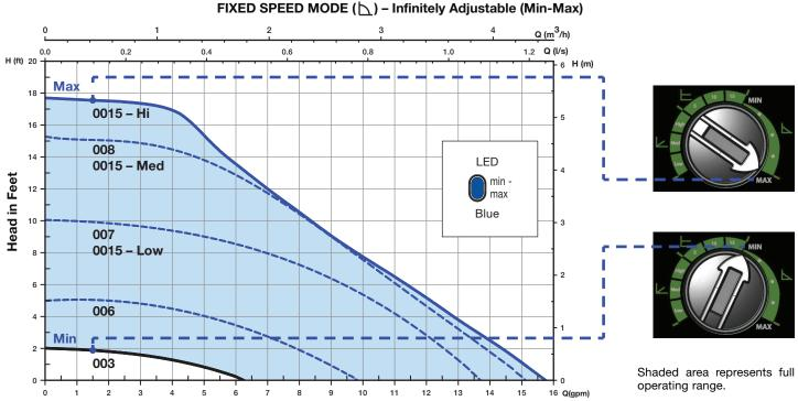
Fixed speed mode ( $\triangle$ ) allows the installer to fine tune the circulator flow rate to precisely match design load conditions. It is infinitely variable between min/max settings. See chart above for equivalent 00 model at each variable speed setting.
