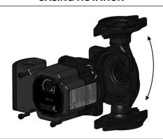
To rotate the casing, remove the 4 motor screws and spin the casing to the desired flow direction. Reattach the 4 screws (\(^{5}\)\_{32}\)"allens wrench required). Be sure body gasket is seated evenly to prevent leakage. Tighten motor screws to 34-42 in-lbs torque.
