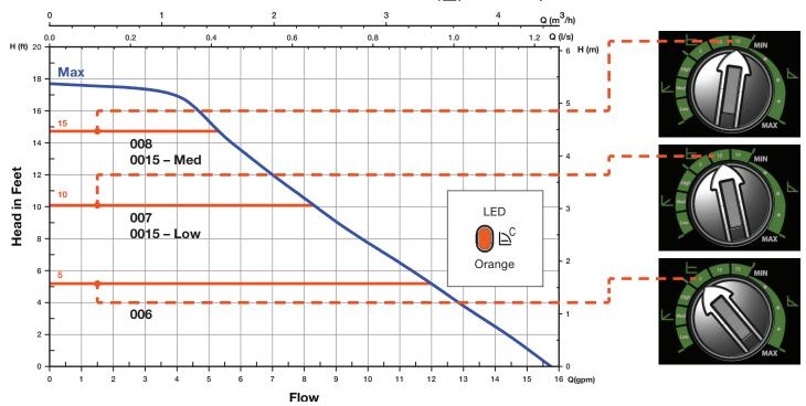
In Constant pressure mode ( $\sqsubseteq$ ), the circulator maintains a constant pressure differential ( $\Delta p$ -c) in the system as heating load increases or decreases. Selection options are 5, 10, or 15 feet of head constant pressure. Seee chart above for equivalent 00 model at each setting.
