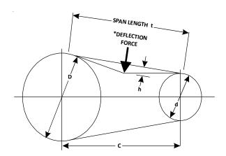
\*Apply force to the center of the span.
