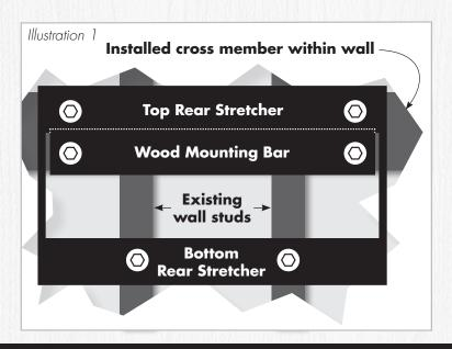
Determine final vanity cabinet top height (excluding counter top) and center, and mark on wall. Measure down  $5\frac{1}{4}$ " to mark where the beveled Mounting Bar top edge will be on your wall
