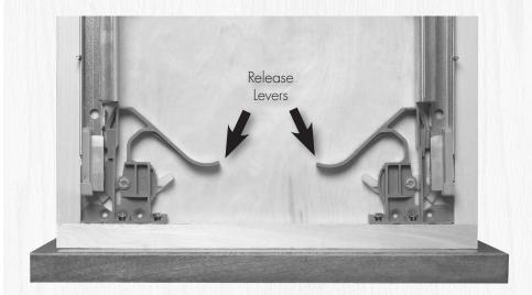
To remove a drawer, open the drawer, reach under it and pull the release levers toward the drawer front. The drawer is now released from the glides. Pull the drawer box toward you and upward to remove.
