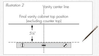
for drilling into wall studs. Drill 3/16" pilot holes into wall and wall studs for 5/16" lag screws. **It is important to drill into stud center.** If installing an ensemble consisting of multiple components, carefully plan mounting bar placement for all cabinets first.
