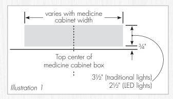
**Traditional lights:** Attach the light housing to the medicine cabinet box securely with screws. Slide the lighting fixture into the housing as shown and secure with the supplied angle pieces.
