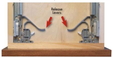
To remove a drawer, open the drawer, reach under it and pull the release levers toward the drawer front. The drawer is now released from the glides and you can toward you and upward to remove.
