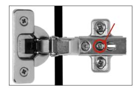
Loosen indicated screw  $\frac{1}{2}$ turn and adjust door in/out. Then tighten.
