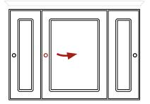
To change the door swing from left-opening to right-opening or vice versa, simple rotate the cabinet body 180 degrees and hang on your wall.
