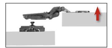
To re-install doors, simply reverse the removal process. Tighten screws part way, adjust door position, and tighten the screws securely.
