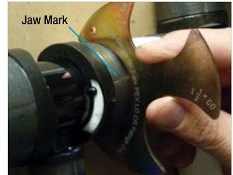
2. The second and slightly smaller opening is to check the crimp ring near the location where the tool jaws meet. At this location, the crimp ring should go completely into the gauge. There are actually 2 diameters near where the tool jaws meet. The crimp is acceptable as long as one of them goes into the gauge.
