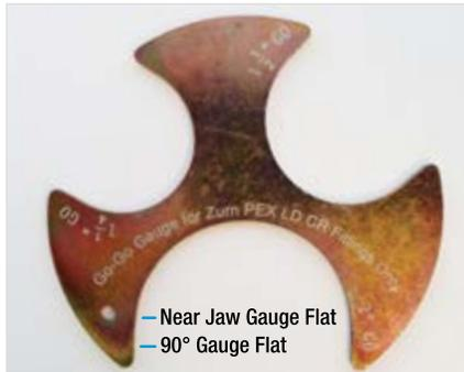
1. For each size of crimp (1-1/4", 1-1/2", 2") there are 2 gauging dimensions. The first and largest opening of each size is to check the crimp ring at 90° to where the tool jaws meet. The gauge 90° opening should go across the mid-point of the crimp ring.
