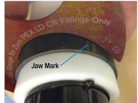
3. If a crimp should not pass the Go-Go Gauge check, it may be re-crimped. We recommend that you try to place the tool as close to the original position as possible, and leaving the tool closed for 15-30 seconds before removing the tool.
