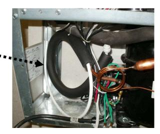
For <u>split level</u> "Versafiller ready" coolers, the tube to plumb in the Versafiller is packaged in the dummy unit.
