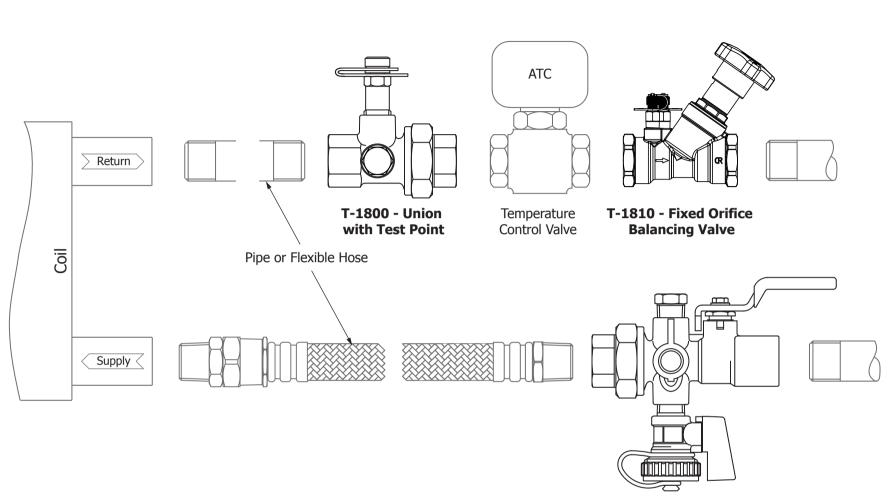
T-1830 - Combination Ball Valve with Drain and Test Point
