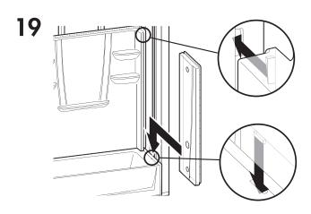
Slide right side wall into position. Be sure locking mechanism is engaged. **NOTE:** Finish caulking is not required, however, if using caulk, weep channel must remain clear of obstruction to allow for proper drainage of the unit.
