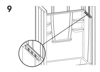
Check for level. Shim if necessary.
