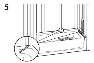
Level and mark all sides. Front apron should be firmly on the floor.
