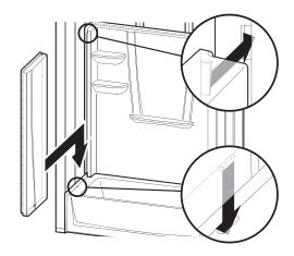
Slide left side wall into position. Be sure locking mechanism is engaged. **NOTE:** To accommodate any stud variation, you may have to add a bead of waterproof adhesive such as 100% silicone to eliminate any potential free play.
