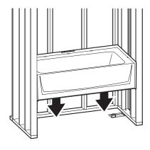
Lift and place the base into framing.
