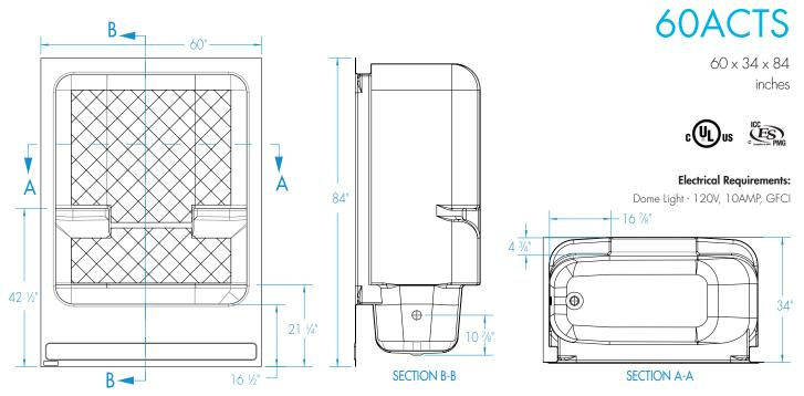
FEATURES lbs Dimensional Tolerance ± 3/8". Dimensions needed for site preparation should be measured from the unit. Aquatic assumes no responsibility for preparatory work.
