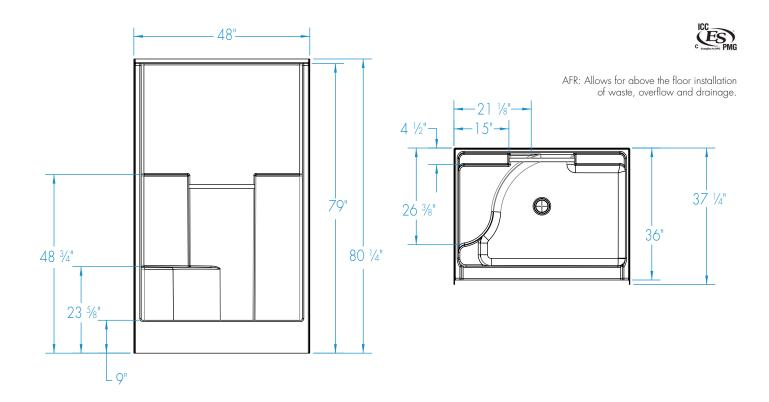
FEATURES Ibs Dimensional Tolerance ± 3/6". Dimensions needed for site preparation should be measured from the unit. Aquatic assumes no responsibility for preparatory work.
