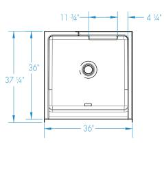
FEATURES Ibs Dimensional Tolerance ± %". Dimensions needed for site preparation should be measured from the unit. Aquatic assumes no responsibility for preparatory work.
