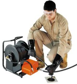
The Foot Pedal interrupts the flow of water between the pump and the nozzle while leaving both hands free to guide the hose. Position the Handy-Reel at the drain site. Connect the jet machine to the inlet on the Foot Pedal. Select and attach nozzle to the hose on the reel. Put the hose 2 to 3 ft. into the drain line. Follow the start-up procedures.
