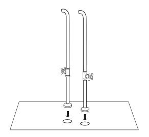
2B. Apply plumber's tape or thread sealant to the threaded outlets on the back of the faucet body. Attach the faucet to the installed supply lines. Tighten firmly using an adjustable wrench.
