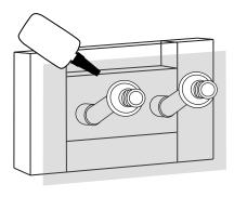
3D. Apply plumber's tape or thread sealant to the threaded outlets on the back of the faucet body. Attach the faucet body to the installed wall mount couplers. Tighten the lock nut firmly using an adjust able wrench.
