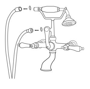
3. To complete the installation. connect the water supply lines (not included) to the faucet's inlets.
