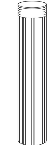
2. Apply plumber's tape to the threading on the tailpiece, then reattach the tail piece to the pop-up drain flange.
