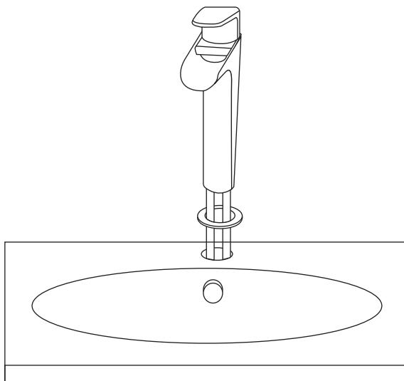
5. From beneath the sink, slide the rubber gasket onto the mounting posts, followed by the metal washer. Ensure that each post passes through its designated hole. Hold in place.
