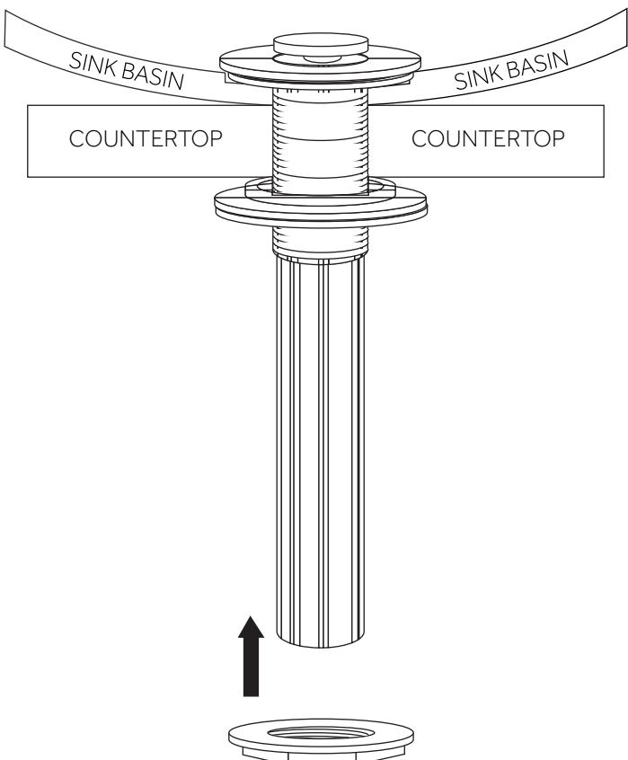
5. From under your counter, slide the tapered rubber gasket followed by the plastic friction washer onto the tailpiece until they meet your sink or countertop. Be sure that the tapered side of the rubber washer is facing up.
