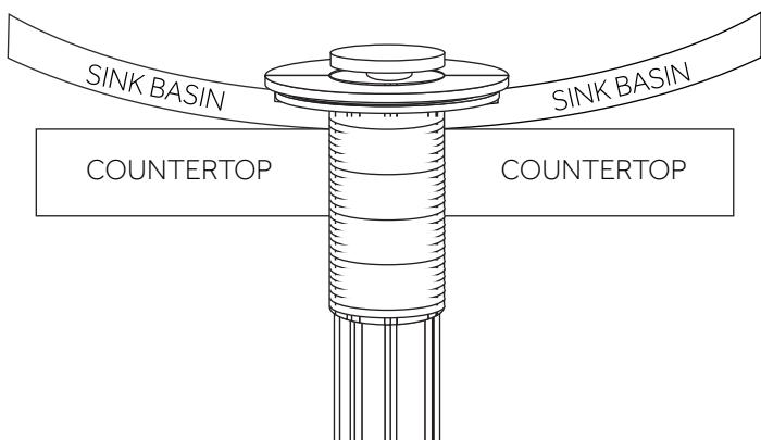
6. Thread the lock nut onto the drain flange. Hand tighten until secure, then finish tightening with a basin wrench once the drain is properly aligned.
