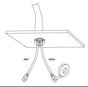
8. Once installation is complete, turn the main water supply back on from underneath your sink. Check for any leaks underneath.
