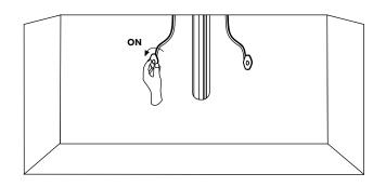
9. Turn the faucet on and ensure that there are no leaks. Check to ensure that both hot and cold water are running properly. Allow the water to flow for approximately 60 seconds to remove any dust or sediment within the water lines.
