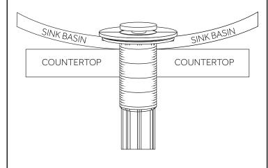
5. From under your counter, slide the tapered rubber gasket followed by the plastic friction washer onto the tailpiece until they meet your sink or countertop. Be sure that the tapered side of the rubber washer is facing up.
