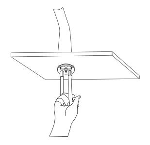
7. Apply plumber's tape or thread sealant to the threading on each braided water line. Attach the water lines to your main water supply lines. Ensure that you are connecting the hot and cold lines appropriately.
