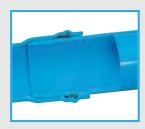
The gasket shall be carefully fitted to the bell groove if not already factory installed. Both bell and spigot shall be clean and free of debris before approved lubricant is applied. The pipe and/or fittings shall be joined by push-fitting bell-and-spigot joint to the depth line marked on the spigot. When pipe has been cut in the
