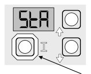
Press "I" key on the control to change from one parameter to the next. Each setting will alternate between display code (for example 5ER) and value.
