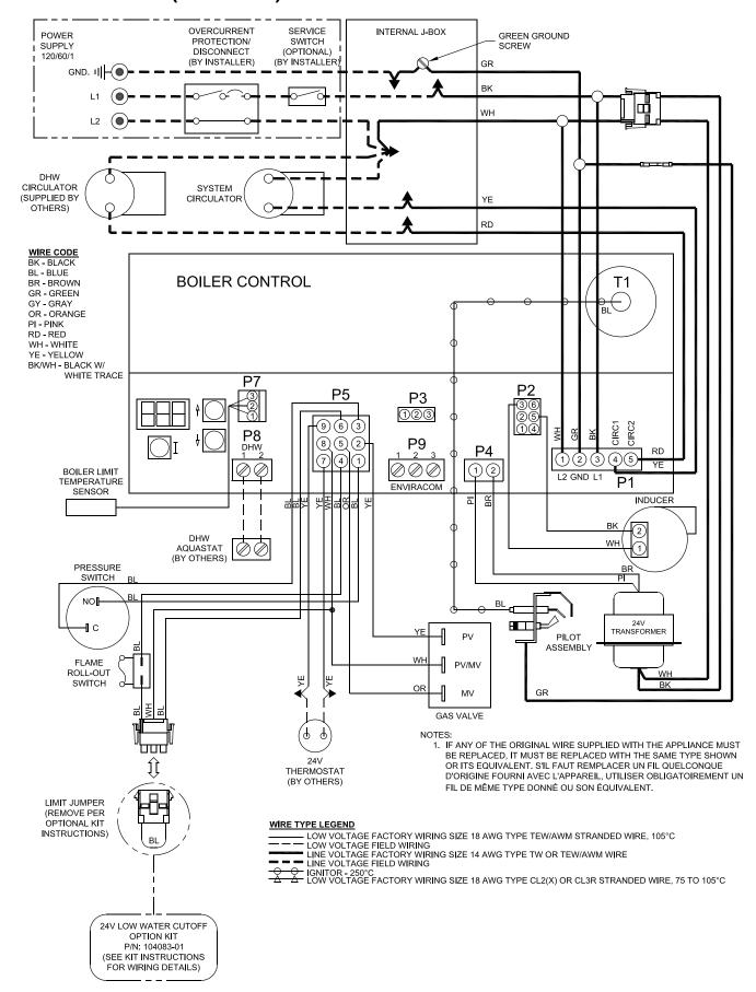
Figure 17: Wiring Connection Diagram
