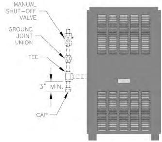
Figure 16: Recommended Gas Piping
