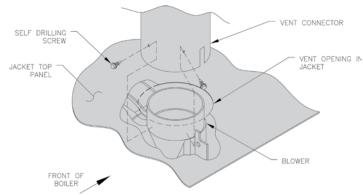
Figure 28: Blower Vent Connector Assembly
