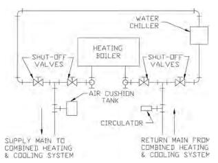
Figure 13: Recommended Piping for Combination
