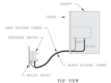
Figure 27: Silicone Tubing Assembly
