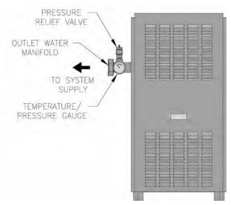
Figure 12: Supply Water Manifold Piping
