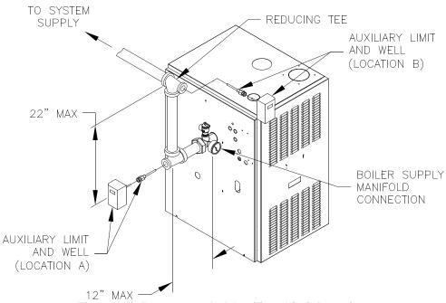
Figure 11: Recommended Auxiliary Limit Location
