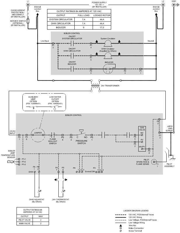
Figure 18: Wiring Ladder Diagram
