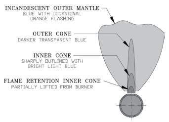
Figure 23: 1 Inch Main Burner Flame
