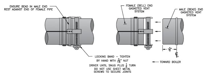
Figure 3: New Yorker Gasketed Vent Joint Detail
