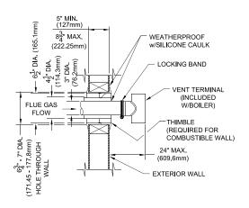
5" MIN. (127mm) 3<u>1</u>" DIA (165 1mm)  $8\frac{3}{4}$ " MAX. WEATHERPROOF (222.25mm) w/SILICONE CAULK 114 3mm) LOCKING BAND VENT TERMINAL (INCLUDED **FLUE GAS** W/BOILER) **FLOW** THIMBLE (REQUIRED FOR COMBUSTIBLE WALL)  $6\frac{3}{4}$ " - 7" DIA. (171 45 177 8mm) E THROUGH 24" MAX. (609.6mm) **EXTERIOR WALL**
