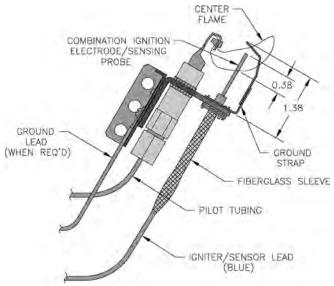
Figure 24: Pilot Burner Flame
