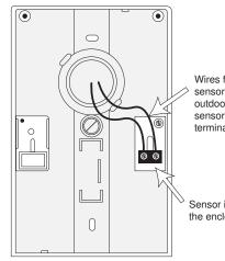
Wires from outdoor sensor to control's outdoor sensor and sensor common terminals
