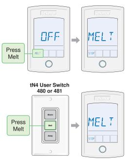
Once manually started, the snow melting system continues to operate until the time set by the Manual Melt Run Time setting in the Set Temp menu elapses.
