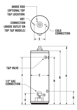
Maximum Hydrostatic Working Pressure: 150 PSI
