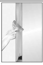
4. Trowel sealant to the desired finish. See tested UL systems for complete installation instructions.
