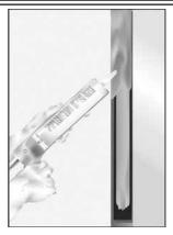
Gun, trowel, or pump approved sealants to minimum 1/4" depth on both sides of wall or top of floor over the backer rod.
