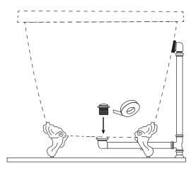
6. To complete installation, reattach the overflow cover plate (**9**) and drain cover plate (**4**) by hand-tightening them from inside of the tub.
