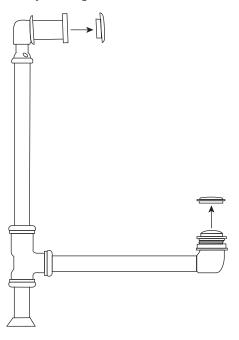
4. **Important**: Do not apply any thread sealant, plumber's tape, or silicone yet. This will be applied later, completing the installation.
