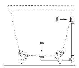
7. Allow the drain to set for 24 hours to allow the silicone and thread sealant to fully dry. Once dry, fill the tub to the overflow point to test the drain and overflow functionallity, and to check for leaks.
