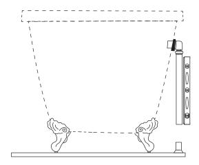
12. The tee connecter (12) will be attached at the points where the drain pipe and overflow pipe intersect. Measure and mark each pipe so that the ends reach a little over halfway into the tee connector's fittings. Ensure that the bottom of the tee connector is properly aligned with the 6" drain piece installed into the floor
