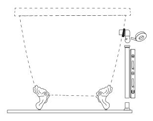
4. Connect the drain pipe (**5**) and overflow pipe (**11**) using the tee connector (**12**). Align the bottom of the tee connector with the installed 6" drain piece (**13**). Once properly alligned, tighten all three slip nuts (**15**) to secure.
