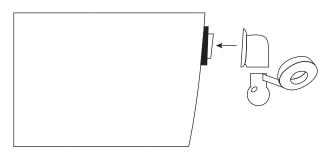
11. Attach the overflow pipe (11) to the ball joint (10) using the attached lock nut. Use a level to align the overflow pipe so that it is perfectly straight, pointing to the floor.
