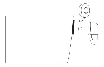
3. Attach the drain pipe (**5**) to the drain elbow (**1**). Apply plumber's tape or thread sealant to the threading before attaching.
