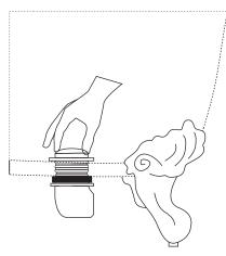
6. Remove the overflow assembly (7) from the overflow elbow (6). Then, remove the overflow pipe (11) from the overflow assembly by loosening the lock nut on the ball joint (10).
