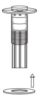
4. Insert the drain flange and tailpiece through the top of your sink's drain hole.
