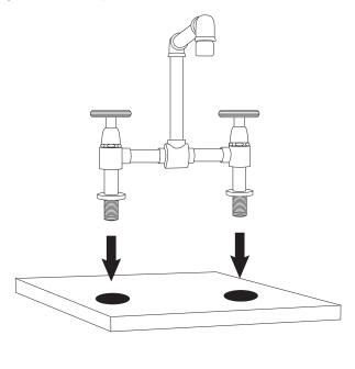
3. From beneath the sink, slide the rubber washers onto the faucet body. Thread the locknuts onto the threaded shanks until hand tight. Finish tightening using a basin wrench.
