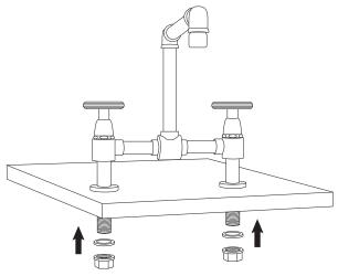
4. Connect the main water supply lines to the faucet. Apply plumber's tape or thread sealant to the threads before tightening. Use an adjustable wrench to tighten, but be careful not to overtighten. Ensure that you are connecting the hot and cold lines appropriately.
