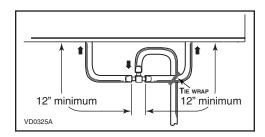
Cut 2 sections of plastic tube, at least 12"-long each, and attach them to each inner drain fitting, located under the unit.
