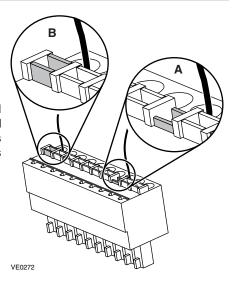
Once the wall control(s) connections have been made, insert the terminal connector in the electrical compartment front face.
