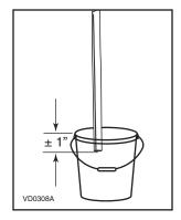
Run the tube to the floor drain or to an alternative drain pipe or pail.
