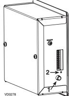
If a problem occurs during the unit operation, its integrated control LED (2) will blink. The color of the blinking light depends on the type of error detected. Refer to Section 9 Troubleshooting on pages 19 and 20 for further details.
