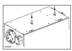
Insert both drain plugs (included in parts bag) in alternate drain fittings located on top of the unit.
