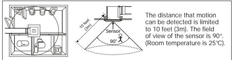
The distance that motion can be detected is limited to 10 feet (3m). The field of view of the sensor is 90°. (Room temperature is 25°C).
