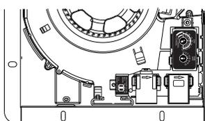
Note that there is ONLY ONE Plug 'N Play slot to insert the Multi-Speed module within the base model fan. There are TWO interchangeable Plug 'N Play slots to insert the Condensation Sensor module, Motion Sensor module within the base model fan.
