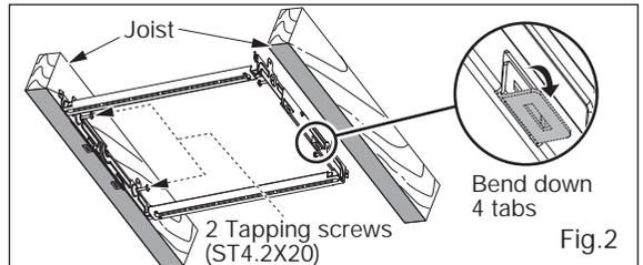
2. Bend down 4 tabs for positioning, install the Flex-Z Fast™ bracket to joists by drilling 2 tapping screws which have been fixed on it. (Fig.2)
