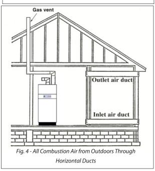
• Where communicating with the outdoors is through horizontal ducts, each opening shall have a minimum free area of not less than 1 sq.in./2000 Btu/hr of total input rating of all equipment in the enclosure. *See Fig. 4 below.*
