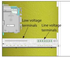
Fig. 20 - Terminal Strip Location
