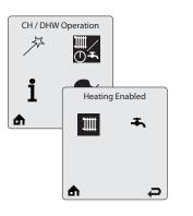
**CH/DHW Operation** provides a simple way to enable/disable either the CH or the DHW function of the HeatMaster TC.
