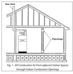
• Combining spaces in different stories. The volumes of spaces in different stories shall be considered as communicating spaces where such spaces are connected by one or more openings in doors or floors having a total minimum free area of 2 sq. in./1000 Btu/hr of total input rating of all gas utilization equipment.
