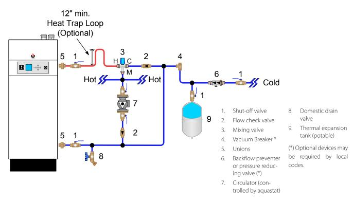
Fig. 7 - Domestic Piping with Optional Recirculation
