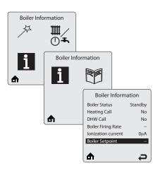
**Boiler Information** provides real time operating information of the HeatMasterTC. Each line contains an information item followed by its current value. Six lines are displayed on the screen at one time.
