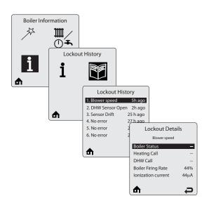
**Lockout History** records the last eight lockouts. Six lines are displayed on the Lockout History screen at one time. Each line contains a lockout description followed by how long ago the lockout occurred.
