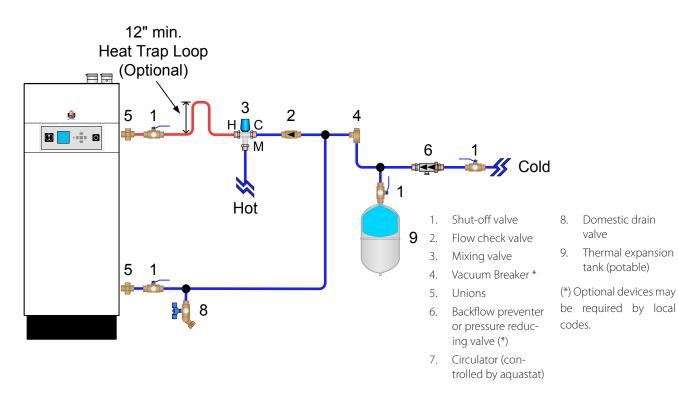
Fig. 6 - Standard Installation Domestic Piping
