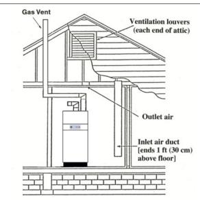
Fig. 3 - All Combustion Air from Outdoors Through Ventilated Attic
