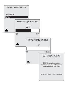
The HeatMasterTC utilizes an Indirect Water Heater sensor. When **Sensor** is selected in Select DHW Demand, use of an Indirect Water Heater Sensor is required. The HeatMasterTC monitors the DHW storage temperature and generates a DHW call whenever the temperature drops below the DHW storage setpoint by 6°F [3°C].
