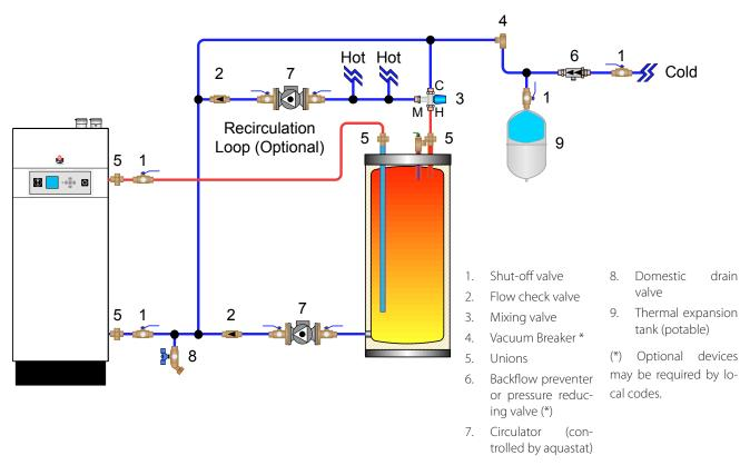
Fig. 8 - Domestic Piping with Optional Storage Tank
