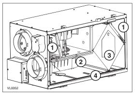
Unit shown in normal position. Can also be installed upside down.
