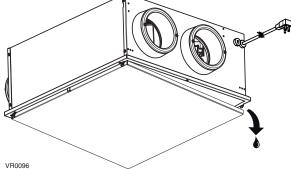
3. While holding the core (1) if unit is installed in or under the ceiling, loosen the wing nut (2) and rotate the core retaining bracket (shaded part in illustration at right). Slide out the core with its filters.
