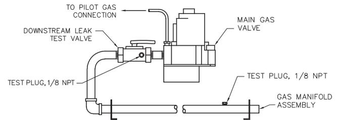
**Figure 5.4: Gas Train Manifold - 64-09 Through 64-12**
