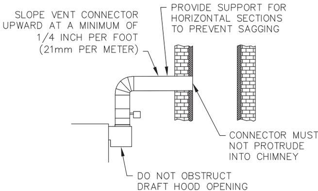
**Figure 3.2: Venting with Vent Damper in Vertical Position**
