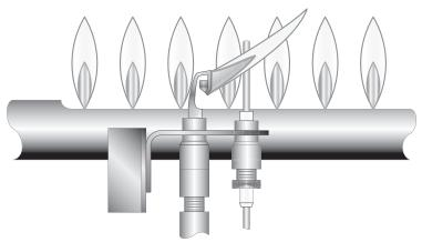
Figure 8.1: Pilot and Burner Flames
