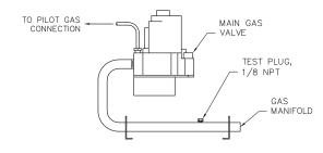
Figure 5.2: Gas Train Manifold 63-03L Through 63-06 8. Typical gas train manifolds are illustrated in Figure 5.2 through 5.4.
