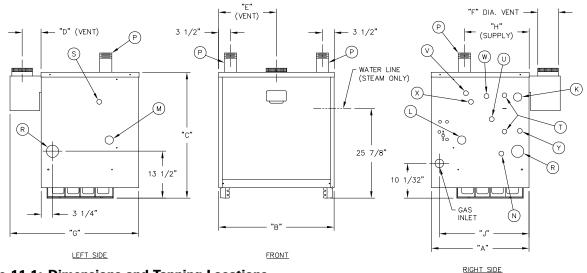
**Figure 11.1: Dimensions and Tapping Locations**
