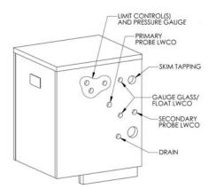
Figure 6.2: Steam Boiler Tapping Location
