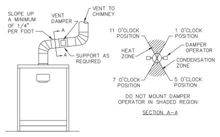
Figure 3.3: Venting with Vent Damper in Horizontal Position
