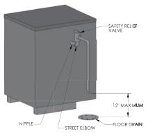
Figure 6.6: Relief Valve Piping Water Boiler
