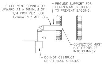
Figure 3.2: Venting with Vent Damper in Vertical Position
