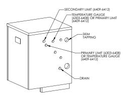
Figure 6.7: Water Boiler Tapping Locations
