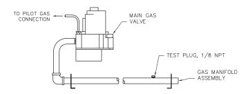
Figure 5.3: Gas Train Manifold - 64-07/08
