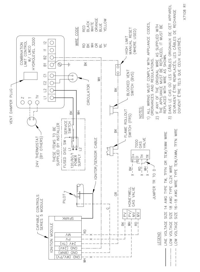
Figure 7.8: Water Boiler with Hydrolevel Hydrostat $^{\scriptscriptstyle (\! 8\!)}$  3200 Limit Control
