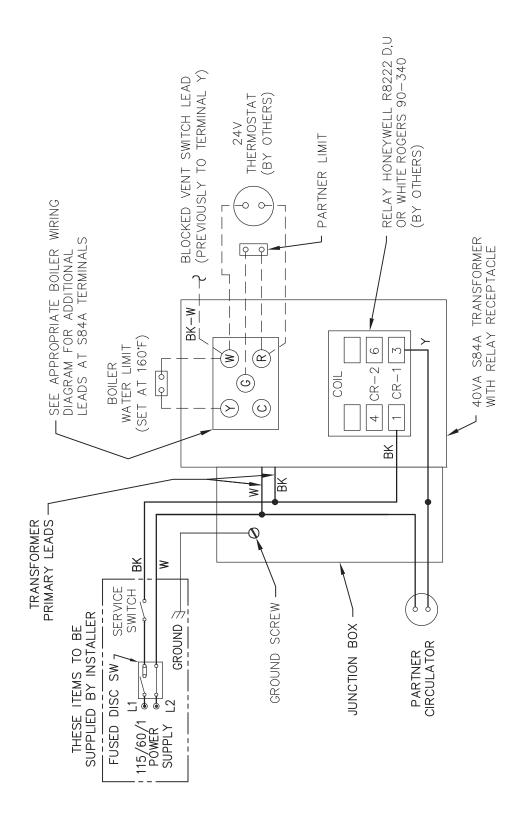
Figure 7.9: Typical Steam Boiler Indirect Water Heater Wiring
