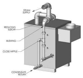
Figure 4.3: Steam Piping – Single Supply Connection
