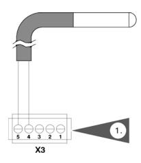
Connect the low-loss header sensor (if LLH is used) to terminals X3.4/X3.5 on the boiler control board.
