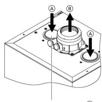
When utilizing the combustion air inlet seal (A) for Vitodens 200 B2HB boilers, remove the inlet seal (A), tear out center section and install the remaining rubber seal back into the air inlet opening.
