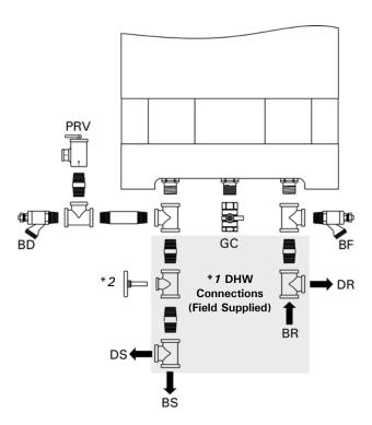
Use an approved pipe sealant or teflon tape when connecting the following installation fittings.
