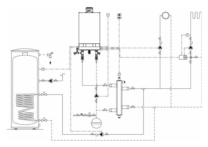
\*Note: When using a low loss header in the system, the DHW connections can be made downstream of the low loss header. See Vitodens 200-W B2HB Service Instructions for applicable system coding information (see coding level 2):
