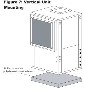
Figure 8: Typical Vertical Unit Installation
