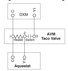
Figure 21: Taco SBV Valve Wiring
