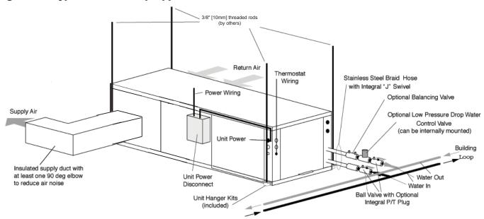
Figure 12: Typical Water-Loop Application
