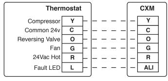
Field Wiring. \_ \_ \_ \_ \_ \_ \_ \_ Factory Wiring.....
