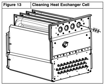
**NOTE**: After cleaning, inspect the heat exchangers to ensure they are free of all foreign objects that may restrict flow of combustion products.
