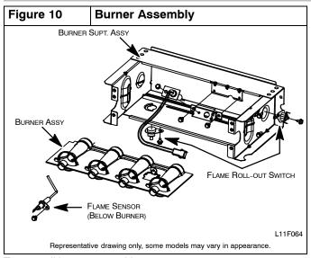
To reinstall burner assembly:
