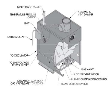
Figure 6.1: Wiring, Controls and Safety Devices
