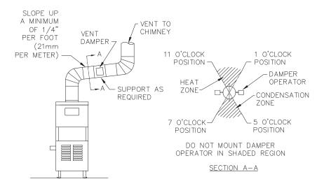
Figure 4.3: Venting with Vent Damper in Horizontal Position
