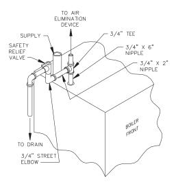
Figure 3.4: Safety Relief Valve Hook-Up with Air Elimination
