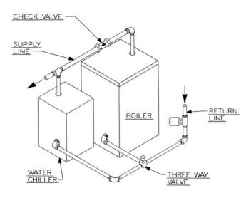
Figure 3.2: Parallel Hook-Up with Water Chiller
