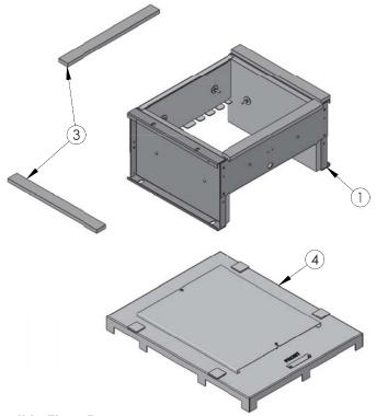
Figure 11.1: Base/Combustible Floor Pan
