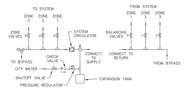
Figure 3.5: Zone Piping with Zone Valves
