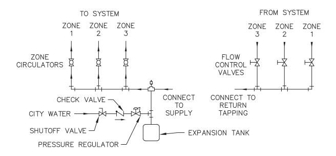
Figure 3.6: Zone Piping with Circulators
