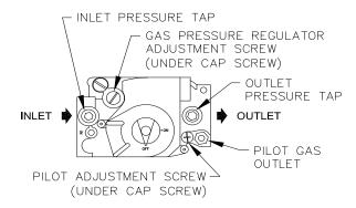
Figure 7.2: Valve Tapping and Adjustment Screw Locations
