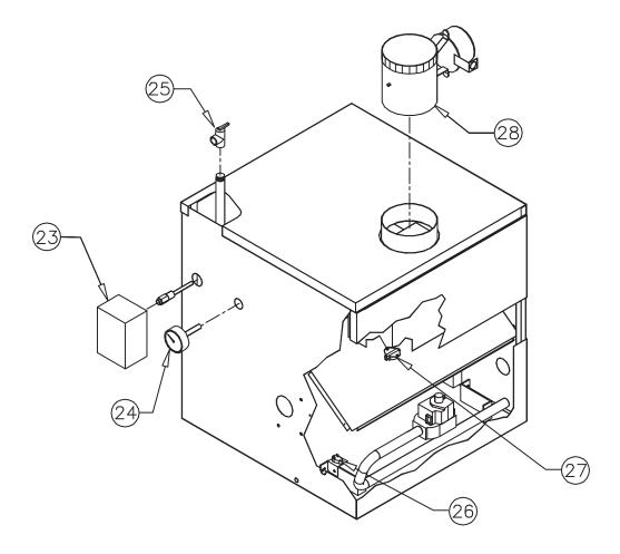
Figure 11.6: Controls/Circulator/Vent Damper
