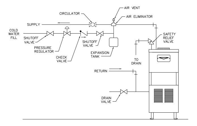
Figure 3.1: Supply and Return Piping
