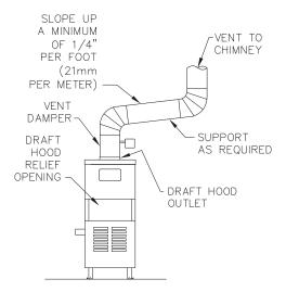
Figure 4.2: Venting with Vent Damper in Vertical Position
