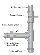
Figure 5.1: Gas Connection to Boiler
