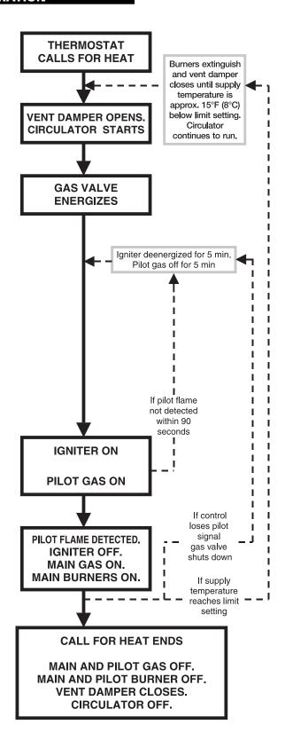
Figure 6.4: Intermittent Ignition System Operating Sequence
