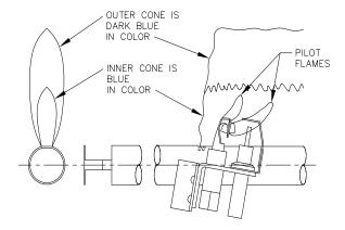
Figure 9.1: Intermittent Pilot and Main Burner Flame
