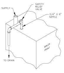
Figure 3.3: Safety Relief Valve Hook-Up Installation with Air Elimination in System Piping
