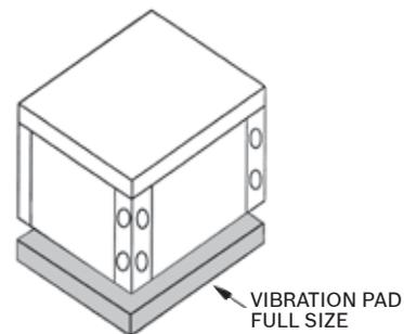
If the unit is installed on a floor over a crawl space, it should not rest on long, unsupported floor joists. Vibrations may be created in the joists with the crawl space acting as an amplifier box resulting in undesirable noise. A drain pan is recommended
