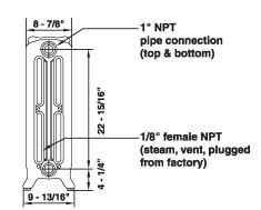
NOTE: Sections use British straight pipe threads and will not adapt to NTP threads without the use of 3/4" or 1" bushing kits
