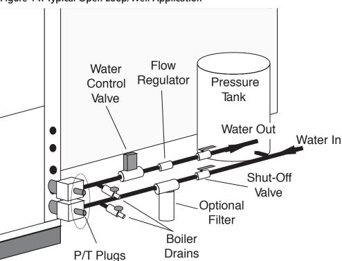
Figure 14: Typical Open Loop/Well Application
