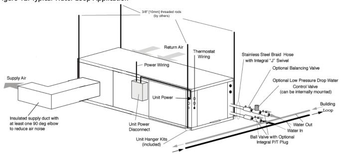
Figure 12: Typical Water-Loop Application
