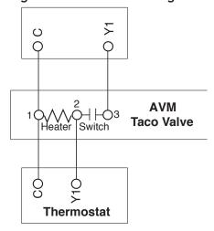
Figure 21: Taco SBV Valve Wiring
