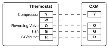
Field Wiring - - - - - - - Factory Wiring -----
