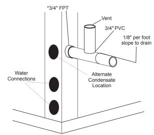
\* Some units include a painted drain connection. Using a threaded pipe or similar device to clear any excess paint accumulated inside this fitting may ease final drain line installation.
