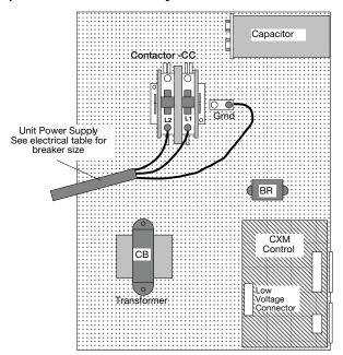
**Power Connection** - Line voltage connection is made by connecting the incoming line voltage wires to the "L" side of the contractor as shown in Figure 15. Consult electrical data tables for correct fuse size.
