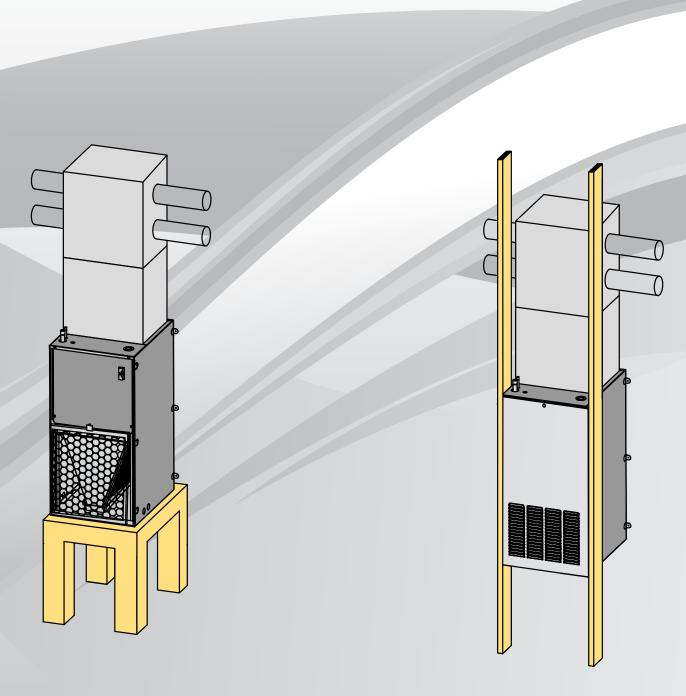
VL\* Air Handler Attached to Back Wall OR Mounted on a Platform in Utility Room VL\* Air Handler Installed in a Stud / Wall Mount Application
