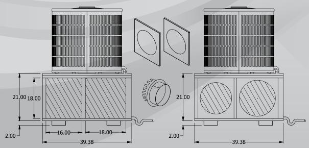
AMCP Units are shipped with round duct adapters installed
