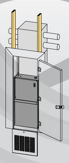
VL\* Air Handler Installed in Closet
