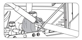
Braze the tubing between the outdoor unit and indoor coil. Flow dry nitrogen into a pressure port and through the tubing while brazing, but do not allow pressure inside tubing which can result in leaks. Once the system is full of nitrogen, the nitrogen regulator should be turned off to avoid pressuring the system.
