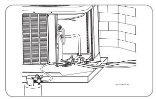
Pressurize line set and coil through service fittings with dry nitrogen to 150 PSIG maximum. Close nitrogen tank valve, let system sit for at least 15 minutes, and check to see if the pressure has dropped. If the pressure has dropped, check for leaks at the line set braze joints with soap bubbles and repair leak as necessary. Repeat pressure test. If line set and coil hold pressure, proceed with line set and coil evacuation (see page 21).
