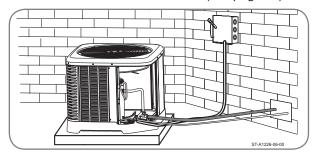
• The vapor line must be insulated for its entire length to prevent dripping (sweating) and prevent performance losses. Closed-cell foam insulation such as Armaflex and Rubatex® are satisfactory insulations for this purpose. Use 1/2" [12.7 mm] minimum insulation thickness. Additional insulation may be required for long runs.
