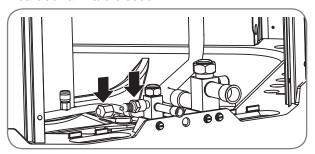
Remove the caps and Schrader cores from the pressure ports to protect seals from heat damage.
