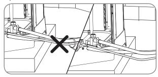
Do not allow the vapor line and liquid line to be in contact with each other. This causes an undesirable heat transfer resulting in capacity loss and increased power consumption.
