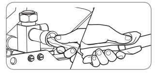
Clean the inside of the fittings and outside of the tubing with a clean, dry cloth before soldering.
