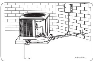
Blow out the liquid and vapor lines with dry nitrogen before connecting to the outdoor unit and indoor coil. Any debris in the line set will end up plugging the expansion device.
