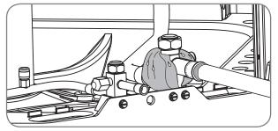
Wrap valves with a wet rag or thermal barrier compound before applying heat.
