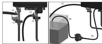
Figure 64 - Flushing the Boiler
