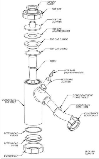
Figure 65 - Condensate Detail
