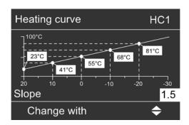
Example: Changing the heating curve slope to 1.5
