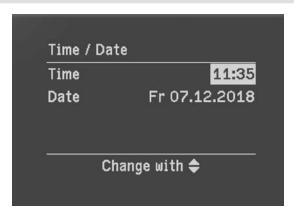
The time and date are factory-set. If your heating system has been without power for a long time, it may be necessary to set the time and date.
