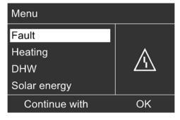
If any faults have occurred in your heating system, the symbol  $\triangle$  flashes in the display, and "Fault" appears. The red fault indicator also flashes (see chapter "Starting the heating system").
