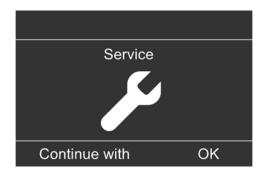
If your heating system is due for a service, the symbol \*Fflashes in the display, and "Service" appears.
