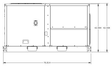
NOTES: 1. THRU-THE-BASE ELECTRICAL IS NOT STANDARD ON ALL UNITS. 2. VERIFY WEIGHT, CONNECTION, AND ALL DIMENSION WITH INSTALLER DOCUMENTS BEFORE INSTALLATION
