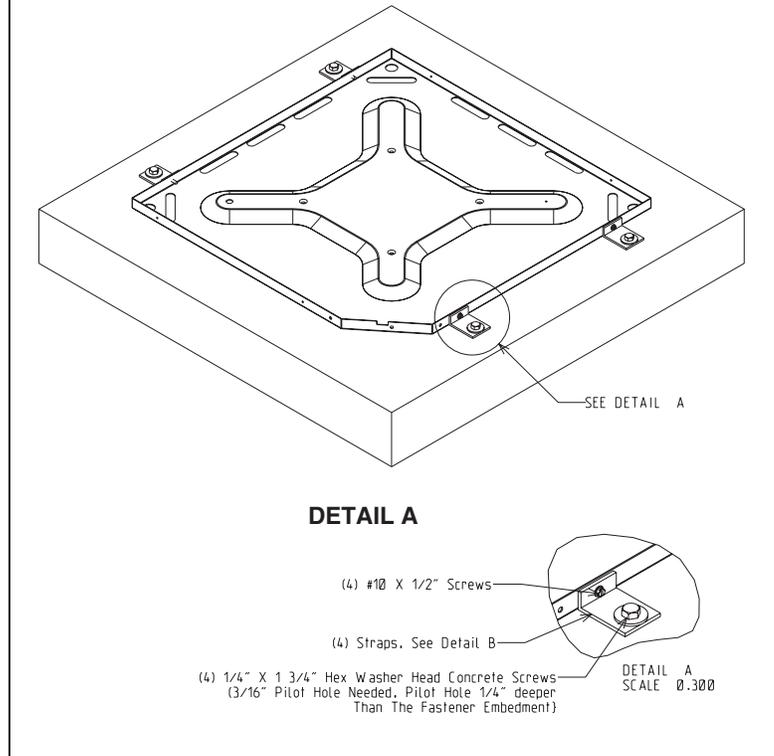
STEP 5: Gauge the amount of washers needed by stacking washers and metal strap in place, as shown in Figure 3, Detail A. Typical installation requires 6 to 7 washers.
