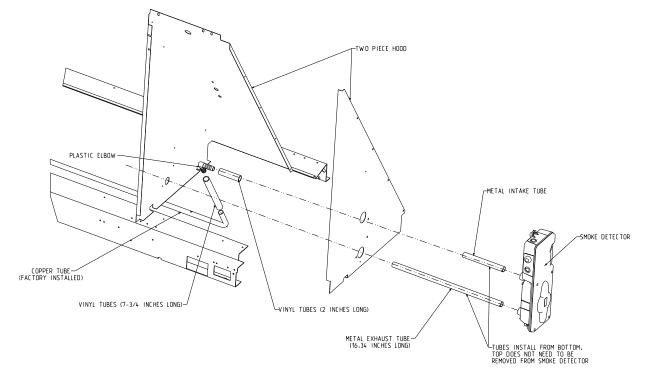
Figure 23. Return air smoke detector for downflow units
