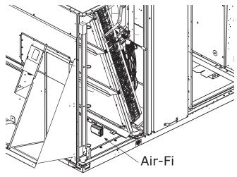
Figure 27. WCI mounting location - WSD150-240 - with low leak economizer
