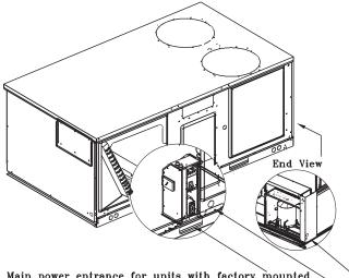
Main power entrance for units with factory mounted disconnect or circuit breaker & GFCI convenience outlet
