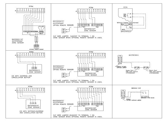
Figure 17. Typical field wiring diagrams for optional controls
