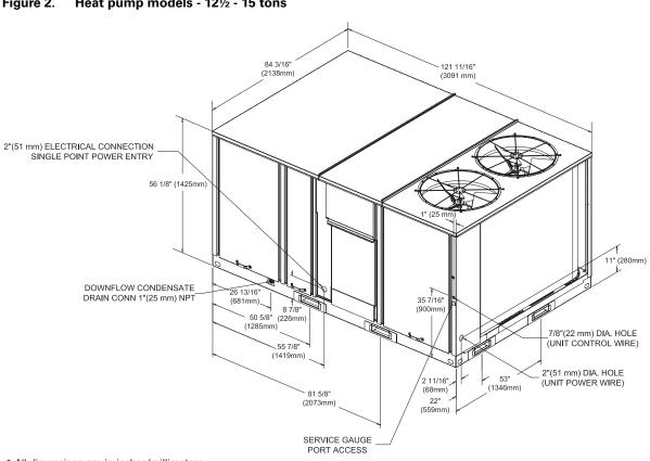
Figure 2. Heat pump models - 121/2 - 15 tons
