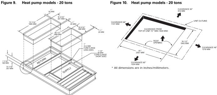
\* Duct flanges mount 7-7/16" down inside the curb on the 1-1½ curb flanges. Roofcurb is intended for downflow use only. \* All dimensions are in inches/millimeters.
