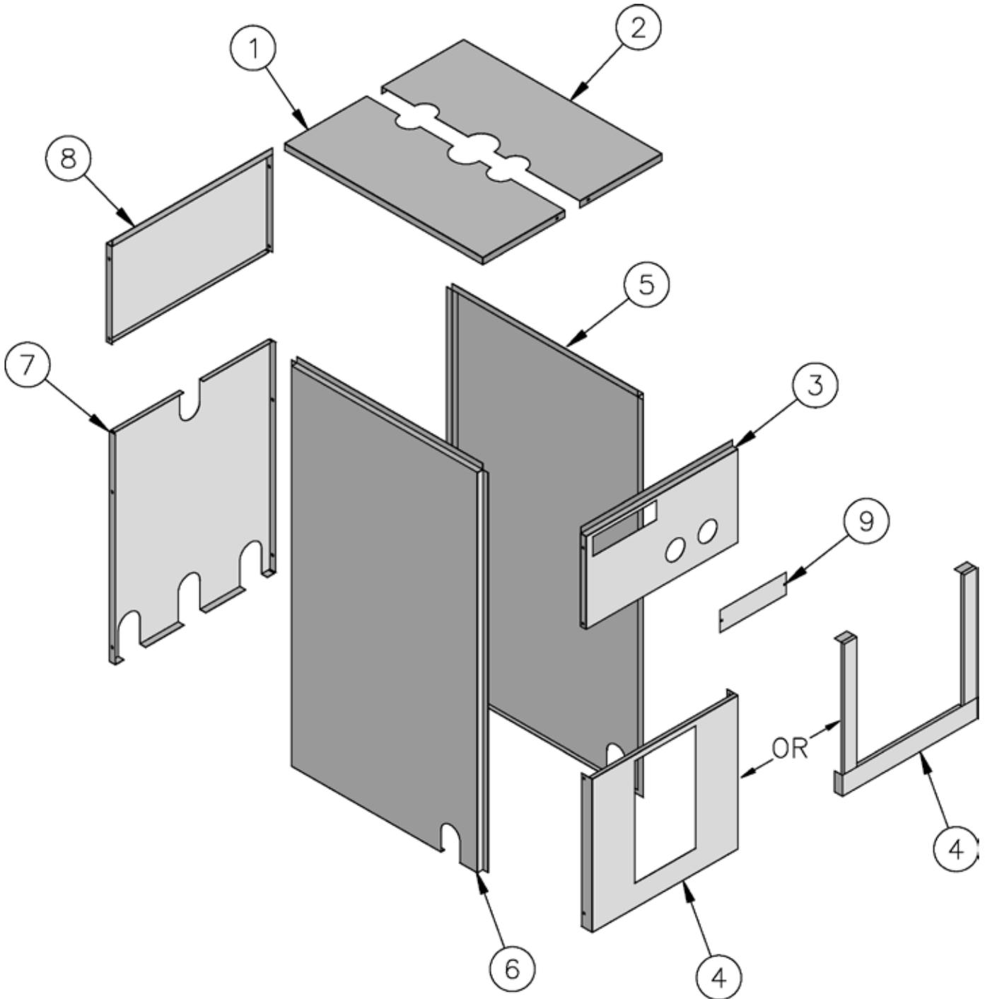
Figure 23: Jacket Repair Parts
