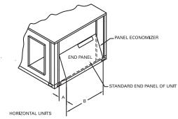
**Note:** When applying economizer to horizontal units, connected ductwork must be run full size to allow proper operation of economizer damper.
