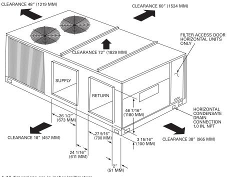
Figure 3. Heat pump models - 121/2 - 20 tons
