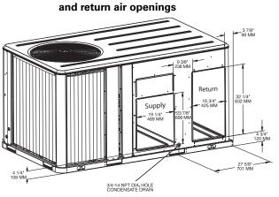
Figure 14. 6 to 10 tons high units-horizontal supply
