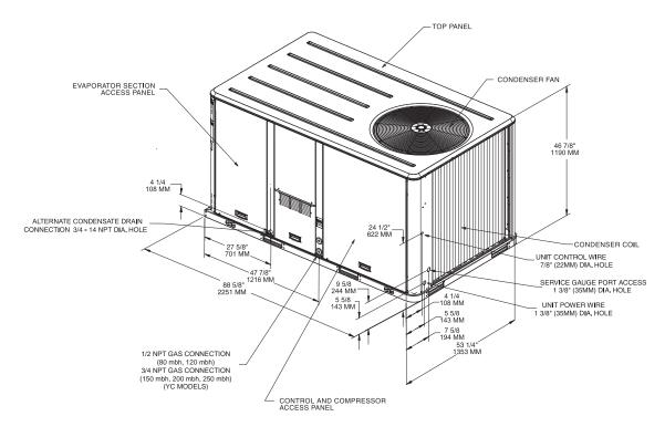
Figure 9. 8½ to 10 tons standard efficiency—roof curb Note: All dimensions are in inches/millimeters.
