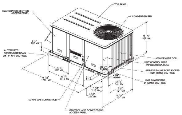
Figure 3. 5 tons standard efficiency-roof curb
