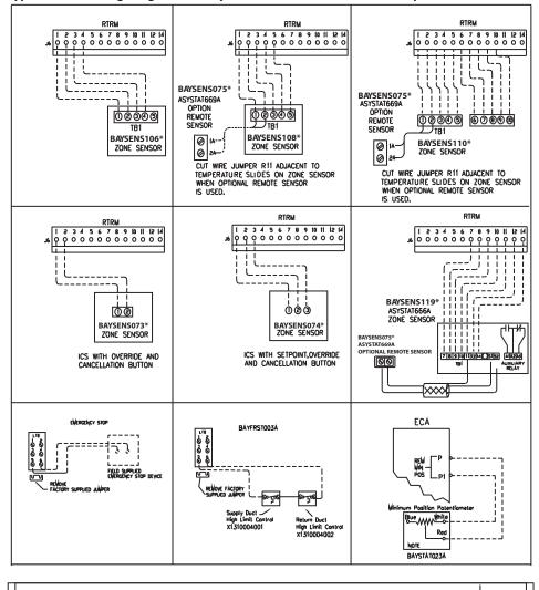
Figure 29. Typical field wiring diagrams for optional controls (ReliaTel<sup>™</sup> only)
