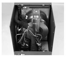
Check the drain connection and drain line to ensure it is clear of debris and sludge. Ensure all hose connections are secure once maintenance of the drain lines is complete.
