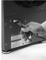
Apply power to DR90/DR120A3000. Turn humidity control to a low RH% to initiate a dehumidification call. Confirm that the compressor and fan turn on. The furnace blower will also turn on to circulate air. Be sure to turn the control to the desired RH% or to Off when the checkout is complete.
