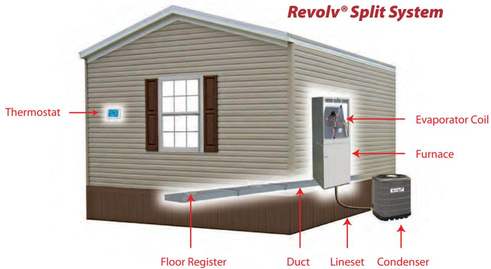
**Revolv Split System** – This describes an air conditioning or heat pump system that is split into two sections - an outdoor section and an indoor section. A typical split system is an air conditioning condensing unit on a pad on the outside of the home, with a furnace or air handler inside the home.
